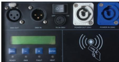
LCD information display area, showing operate menu and working status of machine.
