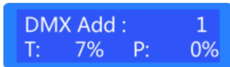
First Line: DMX address, ":" blinks when there is DMX in signal.
